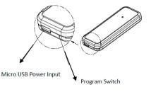
2 For inclusion: Put MyVirtuoso Home gateway into inclusion mode (refer to user manual), press once the program switch on the device to complete the inclusion process. To extend the signal, update the MyVirtuoso Home routing table. To find out how to do this, refer to the gateway manual. For exclusion: Put MyVirtuoso Home gateway into exclusion mode, press once the program switch on the device to complete the exclusion process.
