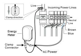
**Note:** If you use the device in a system with photovoltaic plant, the clamp should be placed upstream of the main switch, in order to correctly detect the energy consumption.
